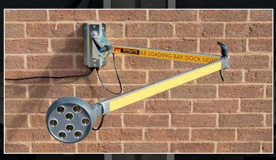
The unit features a rotating variable focusing system that can be adjusted between spot and flood beams for multiple applications, the spot beam enables light to reach further inside container / warehouse area and the light can be focused to ensure minimum glare to workers.
